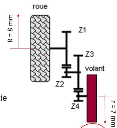
$$\begin{aligned} & \boxed{\begin{array}{l} Z1 = Z3 = 30 \\ Z2 = Z4 = 10 \end{array}} \quad K = \frac{\omega_{roue}}{\omega_{volant}} = \frac{Z4.Z2}{Z1.Z3} = \frac{1}{9} \end{aligned}$$
